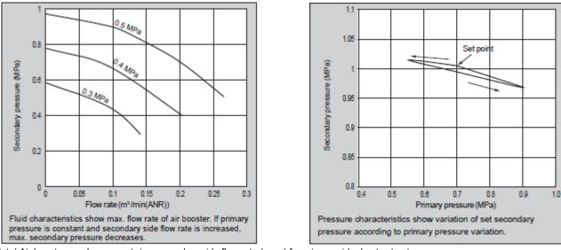
Note) Air booster needs approx. twice secondary side flow rate (max.) for primary side due to structure. Confirm that the instantaneous flow rate is within the curve.
